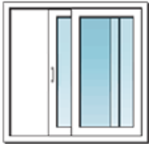
Left Operating Operating / Stationary XO
